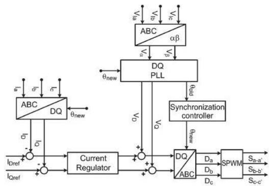
Fig. 2 Block diagram of current controller.
