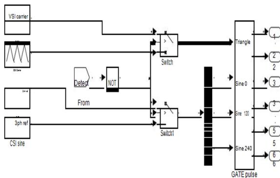
Fig.8 Simulated auto detection and switching in between VSI and CSI modes
