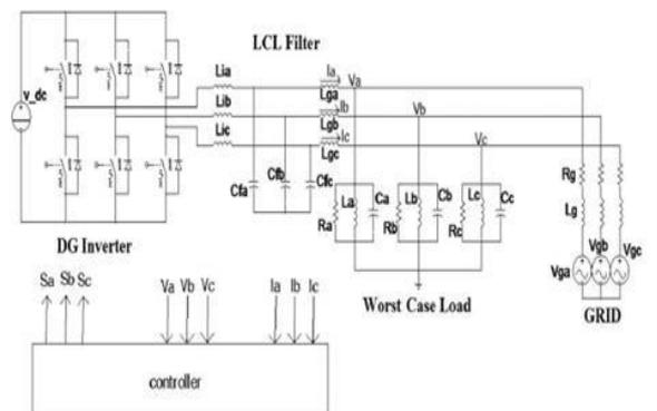
Fig.1 Schematics of DG inverter system
